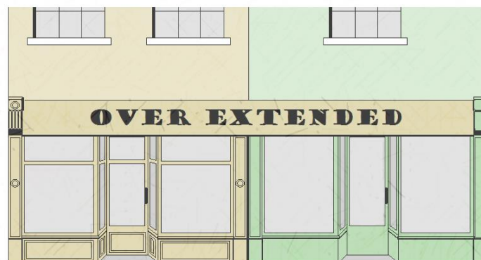
Figure 3: Example where signage has been extended over two units, and appears out of proportion with the host buildings, and obscuring the individual character of each unit.
